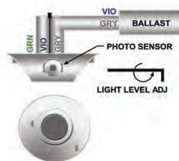
Figure 9.12.3. Photosensor and fluorescent dimming ballast for continuous daylight dimming.
