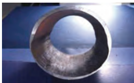
Figure 9.2.13. Condensate pipe – acidic corrosion
